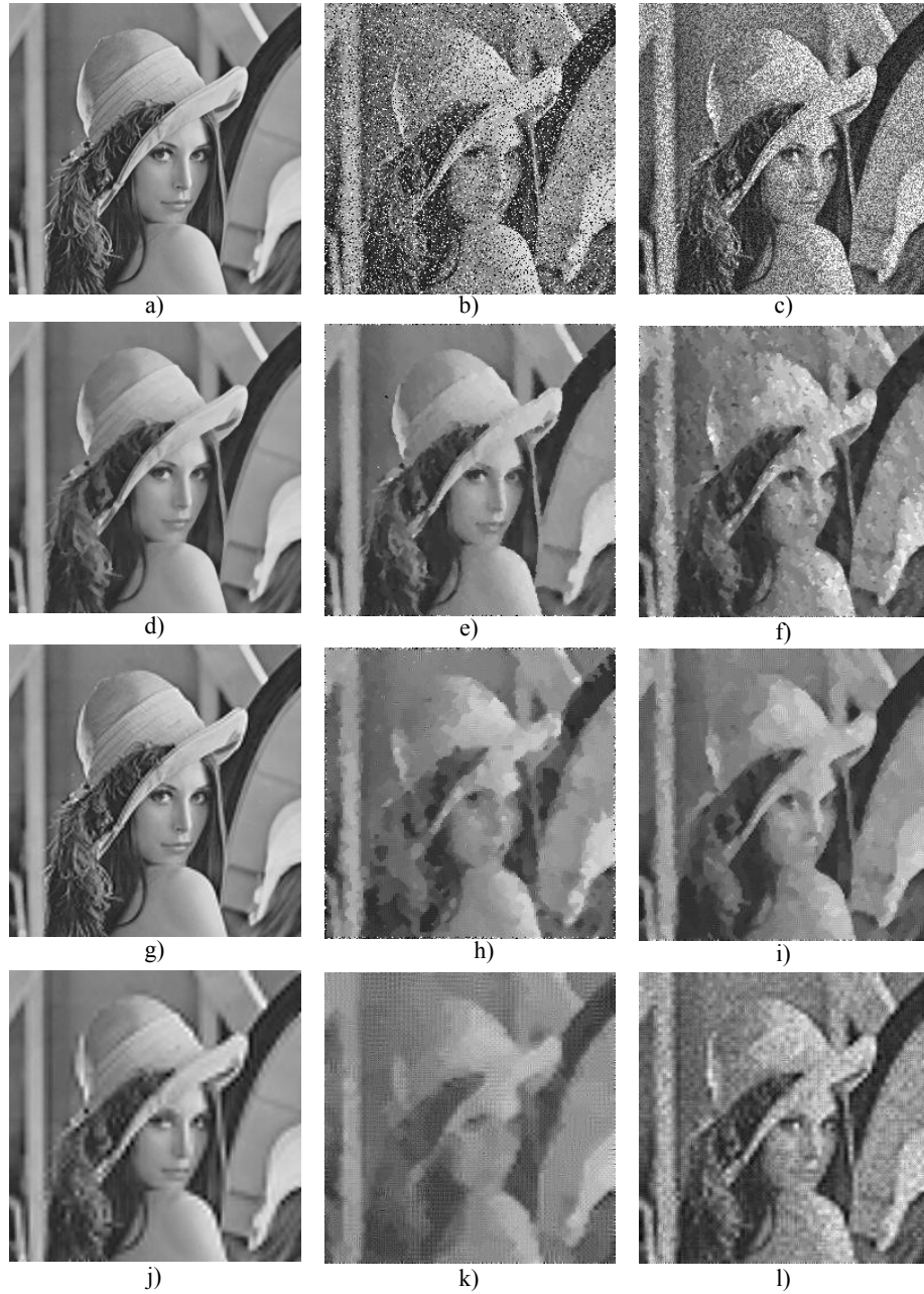
Fig. 2. Visual results in the image Lena, a) Original image, b) Degraded image with 20% of impulsive noise, c) Degraded image with 0.1 of variance of speckle noise, d) Restored image of a) with RM L-filter, e) Restored image of b) with RM L-filter, f) Restored image of c) with RM L-filter, g) Restored image of a) with WDRML filter (db4, D,1), h) Restored image of b) with WDRML filter (db1, A, 1), i) Restored image of c) with WDRML filter (db1, A, 1), j) Restored image of a) with WDRML filter (db3, D,2), k) Restored image of b) with WDRML filter (db3, A, 2), l) Restored image of c) with WDRML filter (db4, A, 2).
